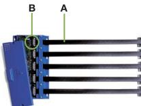
Conventional wire rope inspection relies on time-consuming visual examinations – manually counting surface wire breaks – that take elevators out of service. The Pulse system monitors the electrical resistance of each cord contained in the (A) Gen2 coated-steel belts via (B) conducting pins that penetrate through the belt coating to make electrical contact with each cord. The Pulse monitoring system is installed on all new Gen2 elevators.
