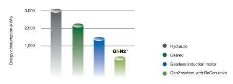
Based on 1000 kg at 1 m/s, 8 stops and 200,000 starts/y (propulsion system only)
