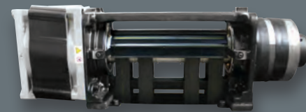
B COMPACT GEARLESS MACHINE Flexible belts allow a smaller sheave, creating a machine that is 70 percent smaller and up to 50 percent more efficient than conventional geared machines.
