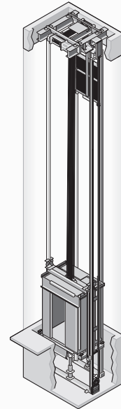
2. CONVENTIONAL MACHINE- ROOMLESS ELEVATOR
